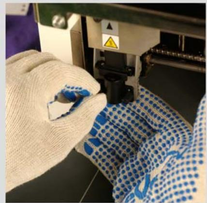
Separate cartridge from machine by removing the two black spindle-screws.
