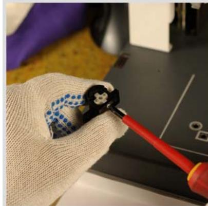
Remove the center screw from black shell. Push up from bottom (pin-side) to remove barrel.
